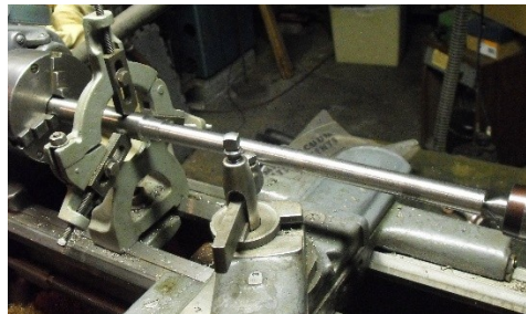
Turning the new stainless shaft on my lathe
