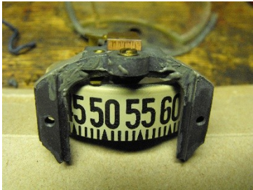
“JB Weld” of broken Drum Yoke legs. Then to be filed to fit. I made a form to fit the bezel in order to re-set the edge over the case flange. Using my lathe and tail center for a work arbor.
