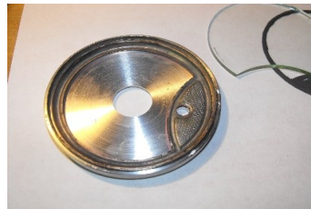
“JB Weld” of broken Drum Yoke legs. Then to be filed to fit. I made a form to fit the bezel in order to re-set the edge over the case flange. Using my lathe and tail center for a work arbor.
