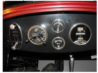
Getting things done on "Remley." New SS water tube. With the rebuilt Speedometer and oil pressure unit "Beulah" now has a full complement of correct gages.
